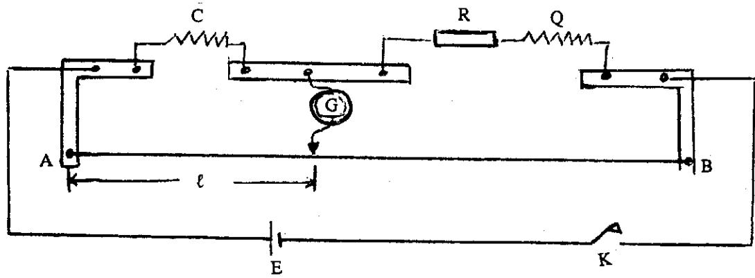
(a) Set up the slide-wire metre bridge as illustrated in the figure above, where C is a standard resistor, R is the resistance box and G is the galvanometer.
