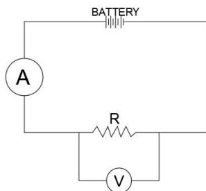
(c) Using the simple electric circuit drawn in 10 (b) above, state the criteria used to connect the ammeter and voltmeter electrical components in the circuit.
