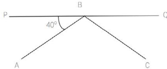
The law of reflection states that the angle of incidence equals the angle of reflection.
